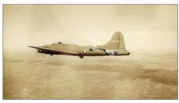
The tail gunner was trapped because there was no floor connecting the tail to the rest of the plane. The waist and tail gunners used parts of the German fighter and their own parachute harnesses in an attempt to keep the tail from ripping off and the two sides of the fuselage from splitting apart.
