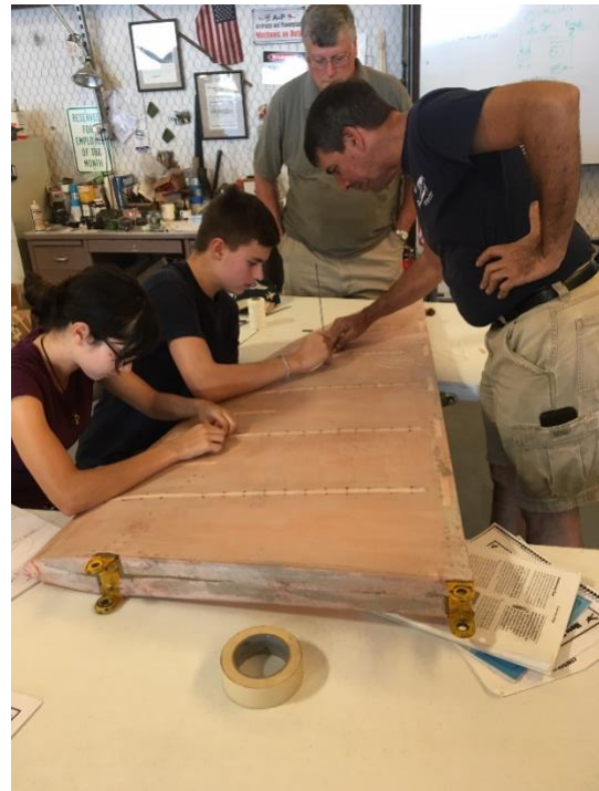
Jim Placette supervises the cadets who are stitching the N3N stabilizer. Photo: Stan Turner
