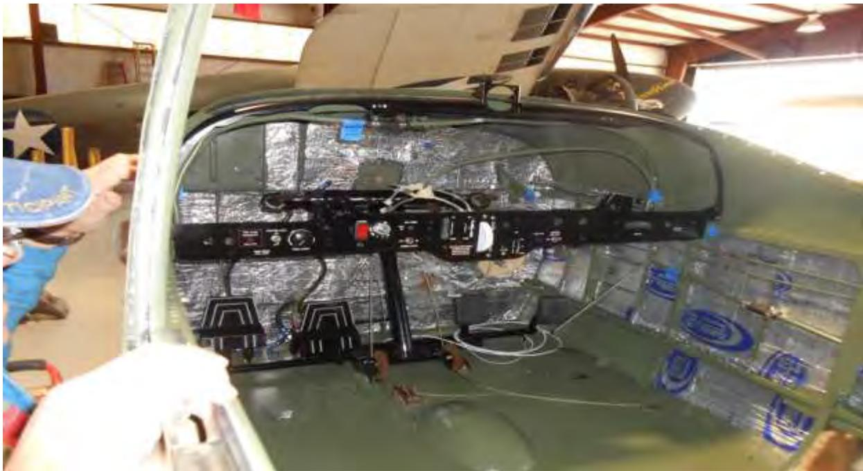
Instrument panel frame installed
